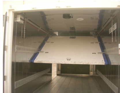
Moveable Partition makes 2 Compartments
