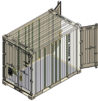
(4) Quadcon Containers coupled together to form one 20' ISO Module
